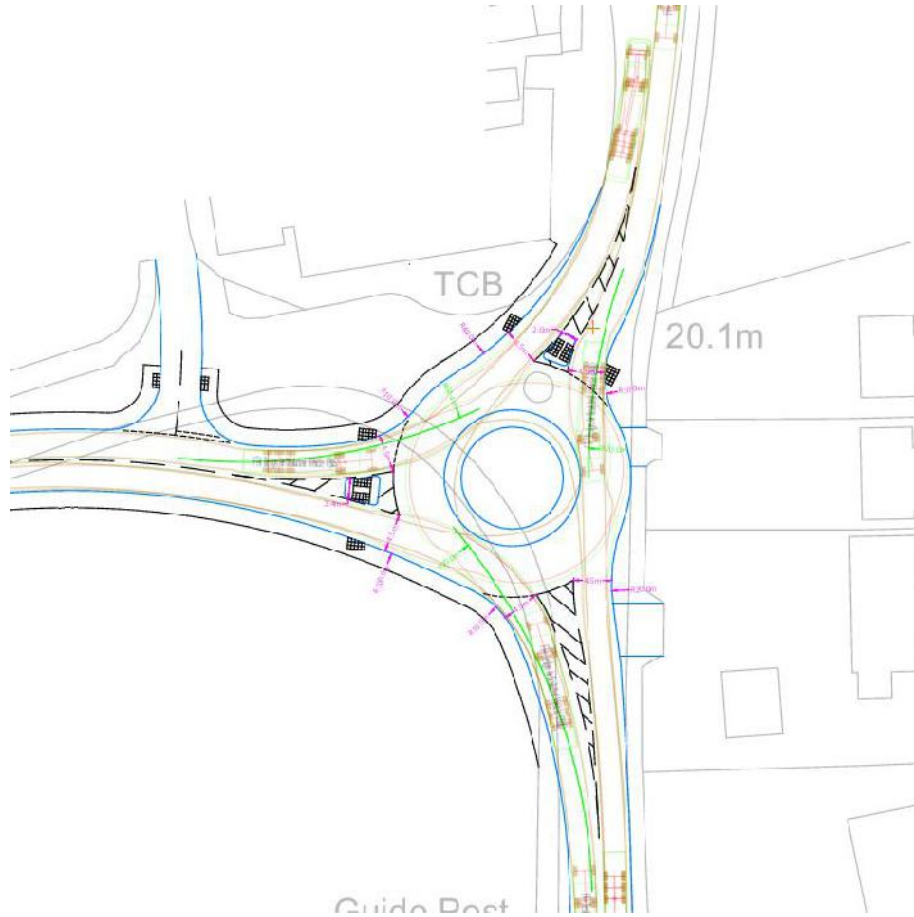
Figure 8.5: A376 / Topsham Road Junction Enlargement
